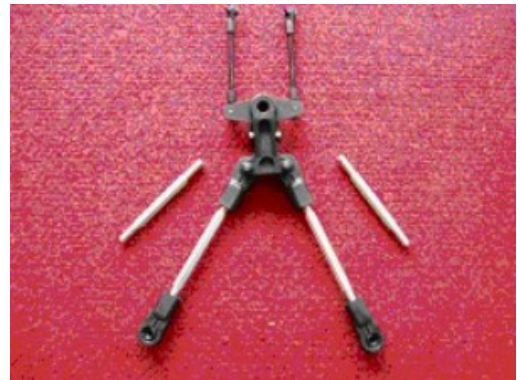
24. Complete steering system and trace pole on the inside drilling of the stub axle mount. See how the ball and socket are flipped to the other side.
